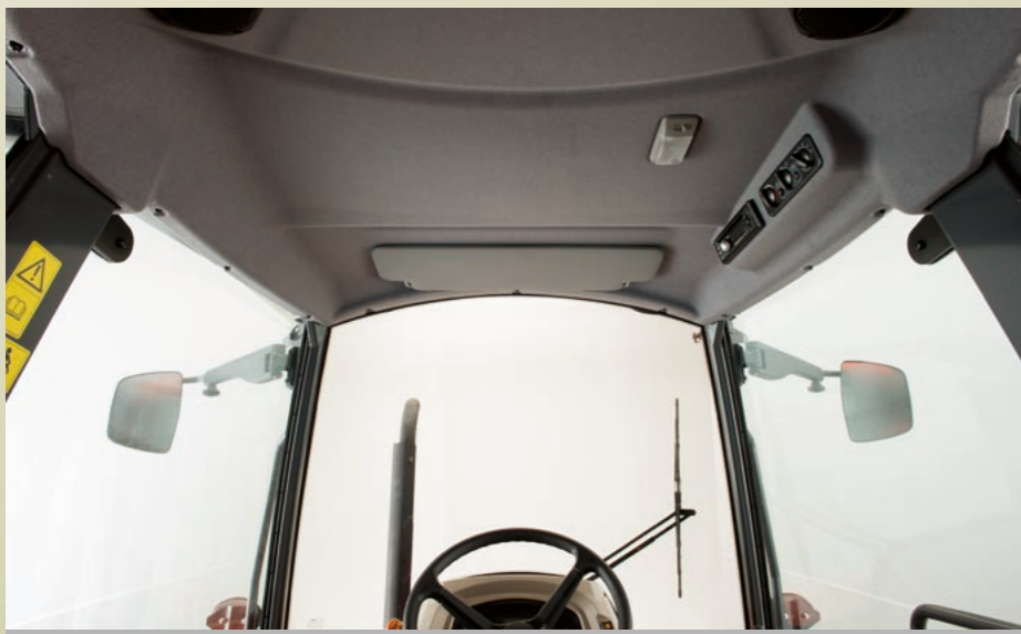
Air is circulated onto the windscreen to prevent icing, frosting and fogging.
