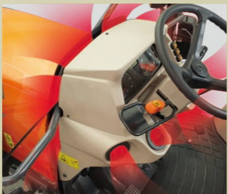
Air is circulated onto the windscreen to prevent icing, frosting and fogging.
